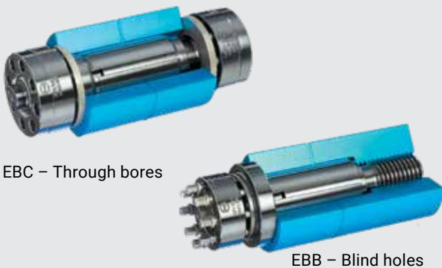
EzFit expansion bolts are radially expanding, axially tensioned coupling bolts. Replacing traditional fitted bolts, which are difficult to install and dismantle, ease of installation and removal is guaranteed. Due to the radial pre-load, the joint experiences an increase in rigidity, therefore eliminating micro-movements on the split flange. EzFit are fully mechanical elements, easy to maintain and are totally re-usable.
