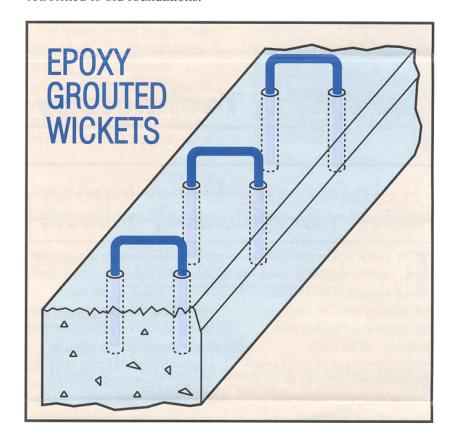
2) Steel added to a deep epoxy grout pour can help bridge hairline cracks in the old foundation below.
