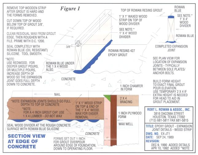
enable the elastomeric seal to go down the sides as well, completing the seal (See Figure 2). After the epoxy grout has hardened, the 1/2" deep removable wood strip is pulled out and any wax cleaned from
