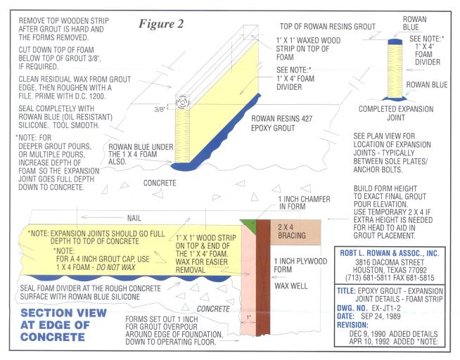
Suitable foam materials of neoprene or urethane are available in 3/4" to 1" width stock. The depth should be approximately that of the grout depth and the length cut to fit
